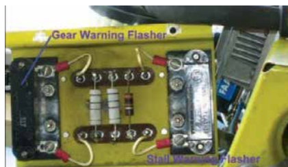
Figure 2: The flasher being used for stall warning and gear warning in the twins. Two resistors have been replaced earlier.
