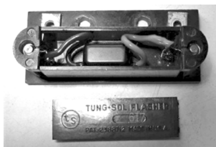
Figure 6: The repair completed with the solid-state flasher circuit inside the original flasher housing lid.
